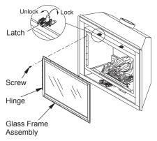
Figure 37 - Removing/Replacing Glass Door
